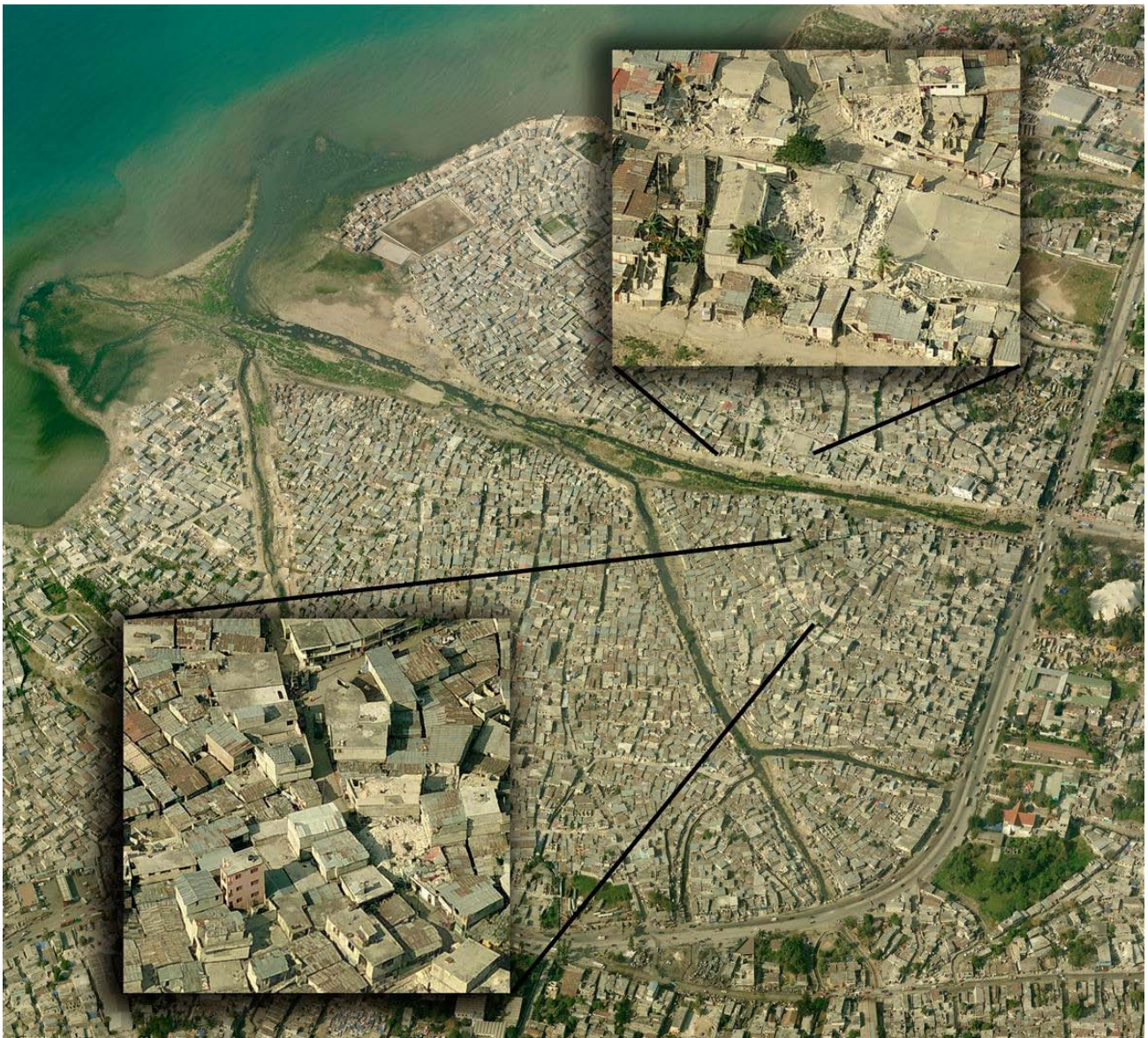
Figure 10. City Eternel an informal settlement on an alluvial fan next to downtown Port-au-Prince, with insets (left) showing 2, 3, and 4 story buildings still standing without visible damage, and only evidence of one collapsed building in the view, and (right) evidence of the collapse of RC frame structures, including an open air market structure among other buildings.
