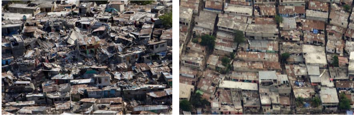
12. Views of bidonville near central Port-au-Prince showing ( left ) view of area with extensive collapses, and ( right ) area with very few collapses. A careful review of the Pictometry of the Port-au-Prince damage district as a whole has shown that views with minimal evidence of collapses was significantly more prevalent than those with heavy collapses. left –UNDP Global (from RMS Report), right © Pictometry
