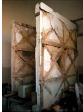
Fig. 17. Gaiola wall sections removed to a government testing lab.
